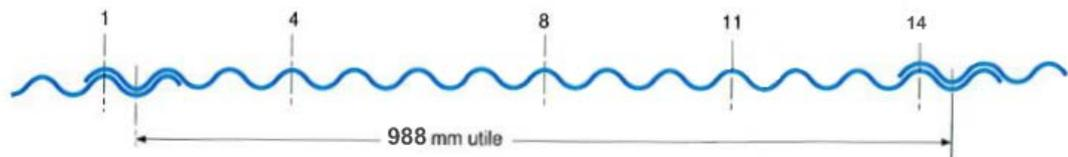
Figure 6 – Fixation des plaques RENOLIT Ondex TO 76 x 18
